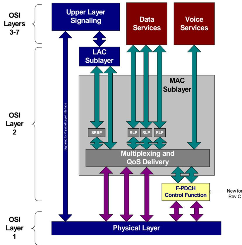
Figure 3. *cdma2000 Rev C Air Interface Layer Architecture*
