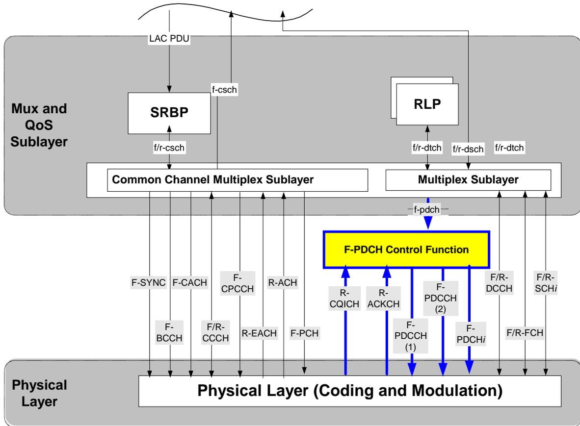
2 **Figure 8. 1xEV-DV Layer 1 Interfaces (Network Perspective)**
