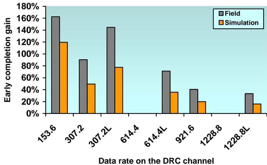
**Figure 8. Early termination gain as a function of data rate.**
