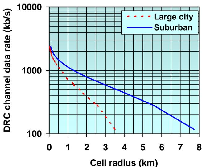
**Figure 11. DRC channel data rate as a function of cell radius.**
