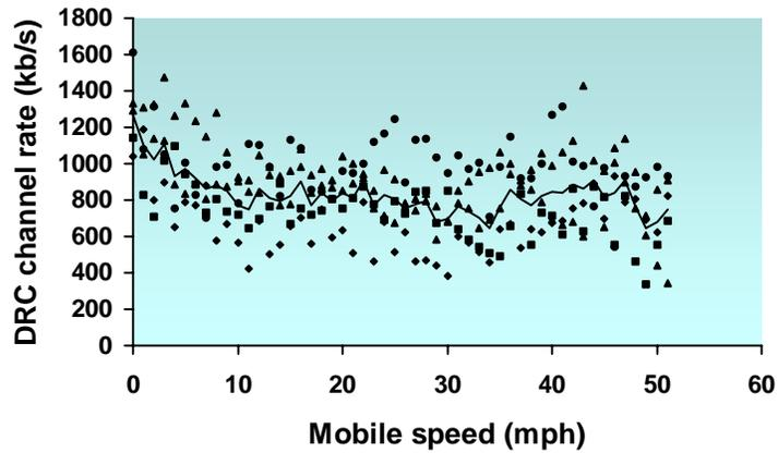
**Figure 6. Data rate measured on the DRC channel as a function of speed.**
