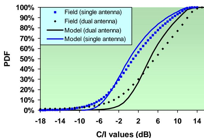
**Figure 3. The  $C/I$  probability distribution function from simulations and measurements.**
