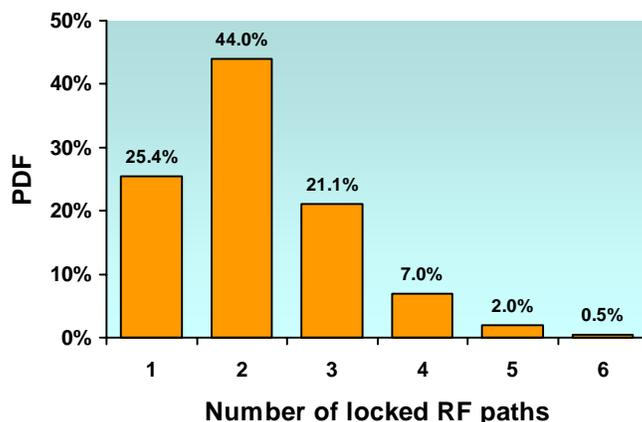
**Figure 4. Number of locked RF paths for the demodulator.**
