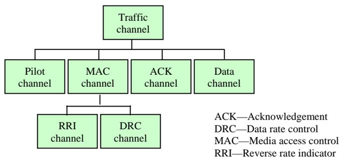
**Figure 1. Reverse link traffic channel structure.**
