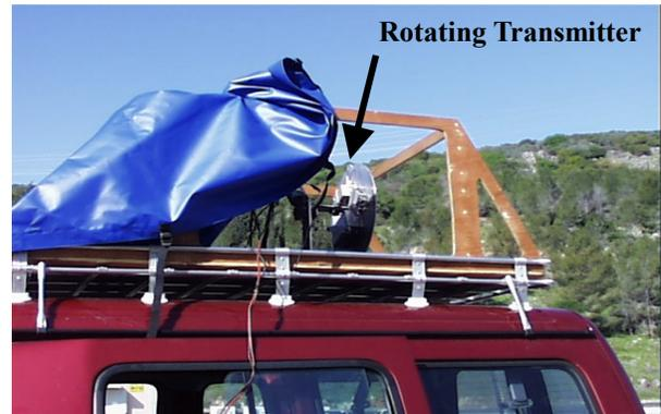
Figure 2: Mobile Transmitter Set-Up
