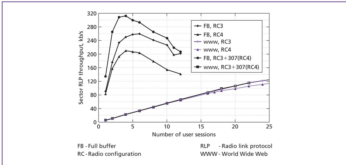
**Figure 4.** Sector RLP throughput as a function of number of sessions using FB and WWW traffic models with RC3 and RC4 and Release 0 and Release A features.
