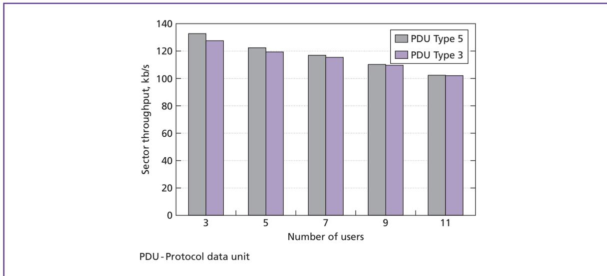
**Figure 2.** Sector throughput as a function of number of simultaneously transmitting users in a mixed-rate system without scheduling gain.
