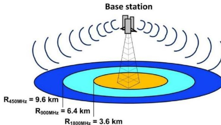
As rule of thumb, a doubling of the spectrum (and therewith a halving of the radio wave lengths) results in a 3-4 times increase in the number of base stations required.
