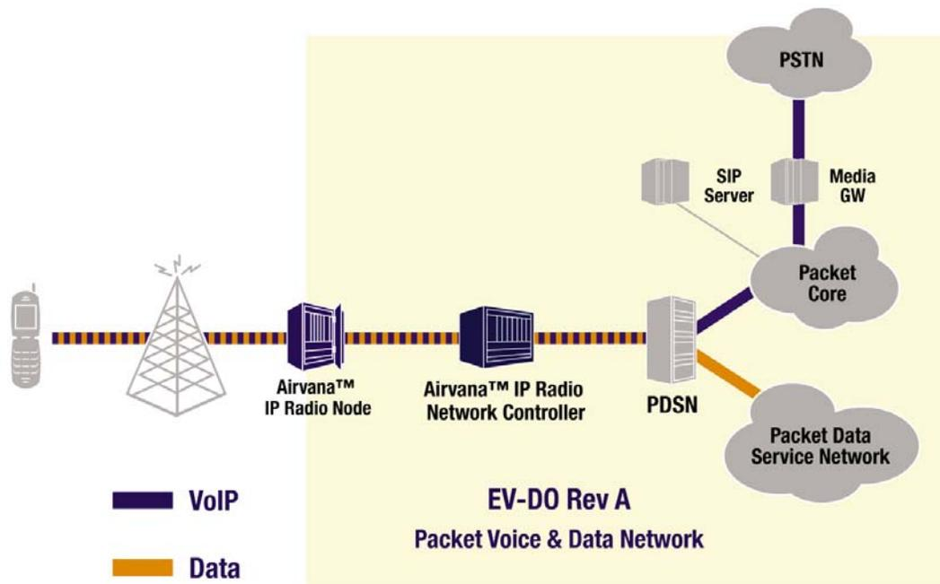
Figure 6: Packet RAN and packet core network
