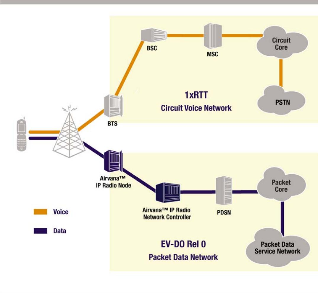
Figure 5: Separate mobile voice and data networks
