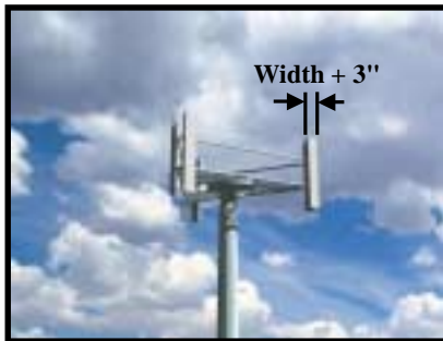
1.9 GHz 4-Branch Intelligent Antenna Spatial Diversity Version
